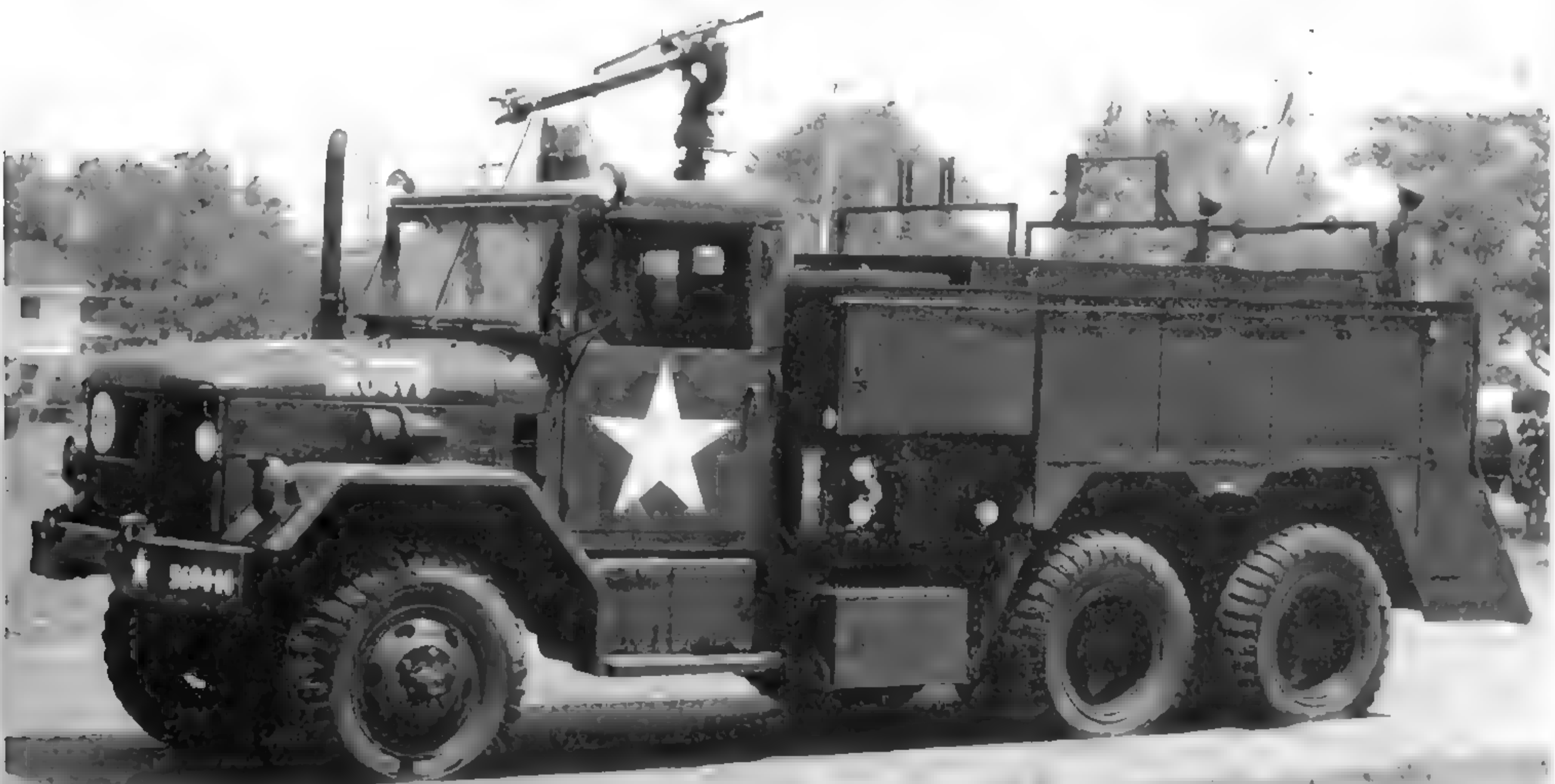
Fire trucks assigned to forward areas were painted in the standard tactical truck paint scheme, as shown here. The widespread use of helicopters in Vietnam spawned the last version of the 530 series, the 530C. The large nozzle on the roof, capable of dispensing foam, was the identifying characteristic of 530C trucks. (Photo courtesy of Richard Adelman collection)
